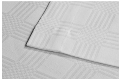
block check dobby weave
